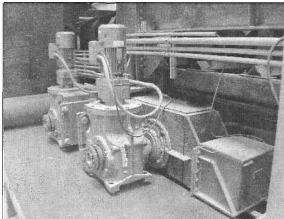
**FIGURE 5 Radomiro Tomić Tripper wheel drives and rail clamp**
