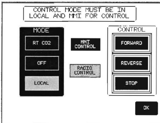
FIGURE 3 Tripper control screen
